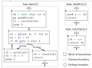
Figure 3: SSA IR built from Listing 1.
