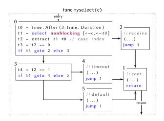
Figure 4: Simplified SSA IR built from Listing 2.
